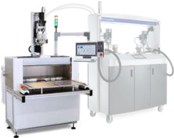
VDS B with Dos P050 dispenser, 2 component, 1 nozzle; LiquiPrep LP804 preparation and feeding unit, 2 component
