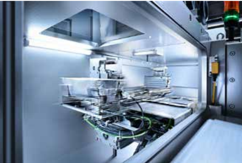
The potting process takes place in the second of the three vacuum chambers. As this chamber is kept under vacuum continuously, short cycle times are guaranteed.
