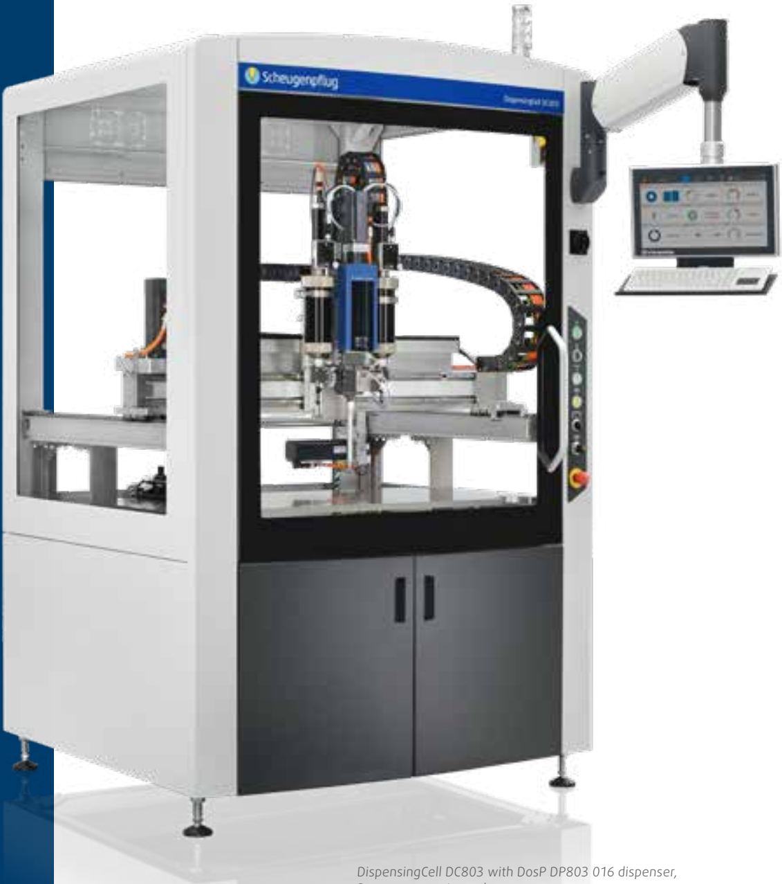
DispensingCell DC803 with DosP DP803 016 dispenser, 2-component, 1-nozzle; two A90 C feeding units
